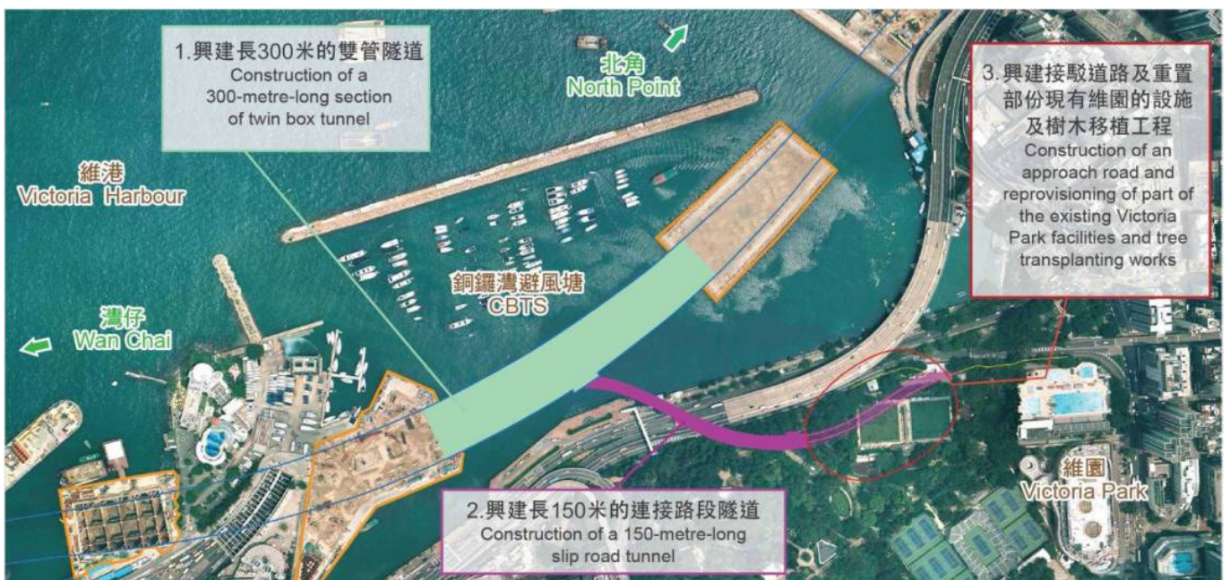
Works under Central-Wan Chai Bypass – Tunnel (Slip Road 8 Section)
