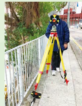
Monitoring survey to track tree displacement
